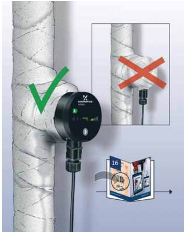
Fig. 5 Insulation of pump housing
